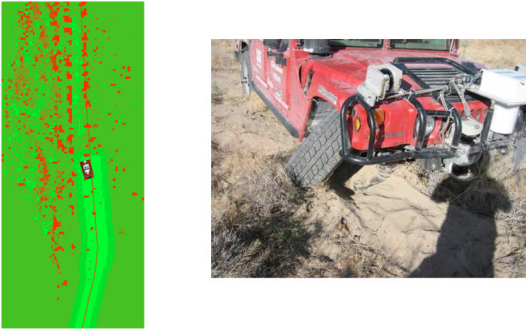
Figure 22. An example of incomplete data (a) which led to significant damage (b). The red continuous line represents the preplanned path. The data show that the preplanned path is on the road edge and veers off the road, which is combined with the hill crest to cause the robot to leave the road.
