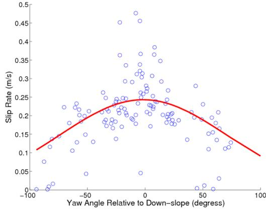
**Figure 5.** Slip rate vs. yaw angle for turning with no plow engaged.
