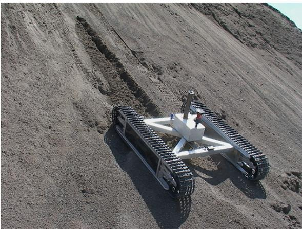
**Figure 10.** Plow engaged during a linear descent, clearly displaying the trench produced as a result of plowing.
