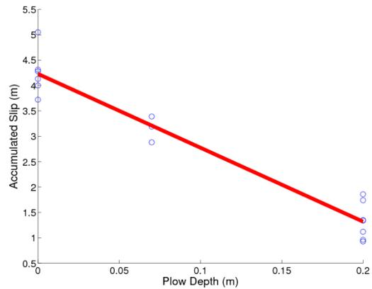
**Figure 4.** Accumulated slip during turning maneuvers with various plow deployments.
