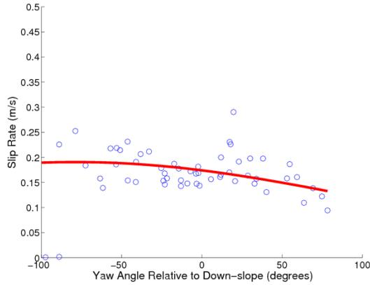
**Figure 6.** Slip rate vs. yaw angle for turning with plow 0.07 m deep.
