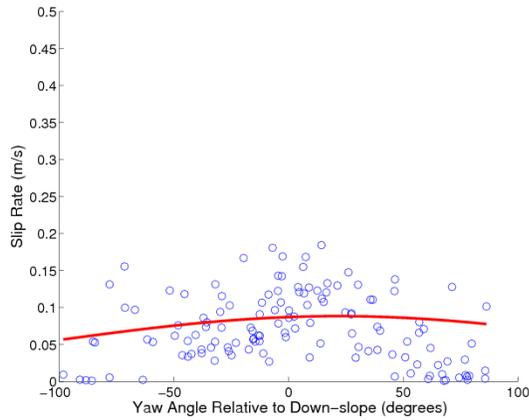
**Figure 7.** Slip rate vs. yaw angle for turning with plow 0.2 m deep.
