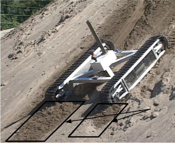
**Figure 9.** Highlighted regions show examples of fluid-like flows of the soil surface layer forming during motion.
