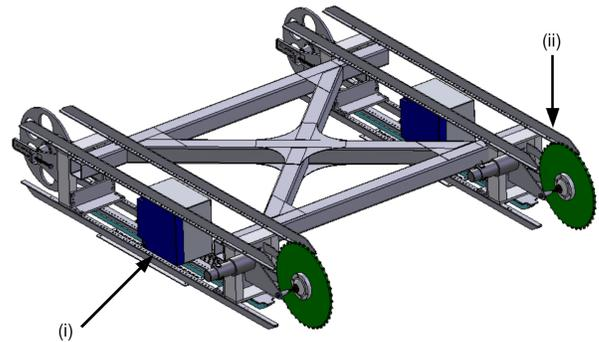
**Figure 1.** Icebreaker chassis design. (i) Internal volume for components (ii) Tracks for locomotion.
