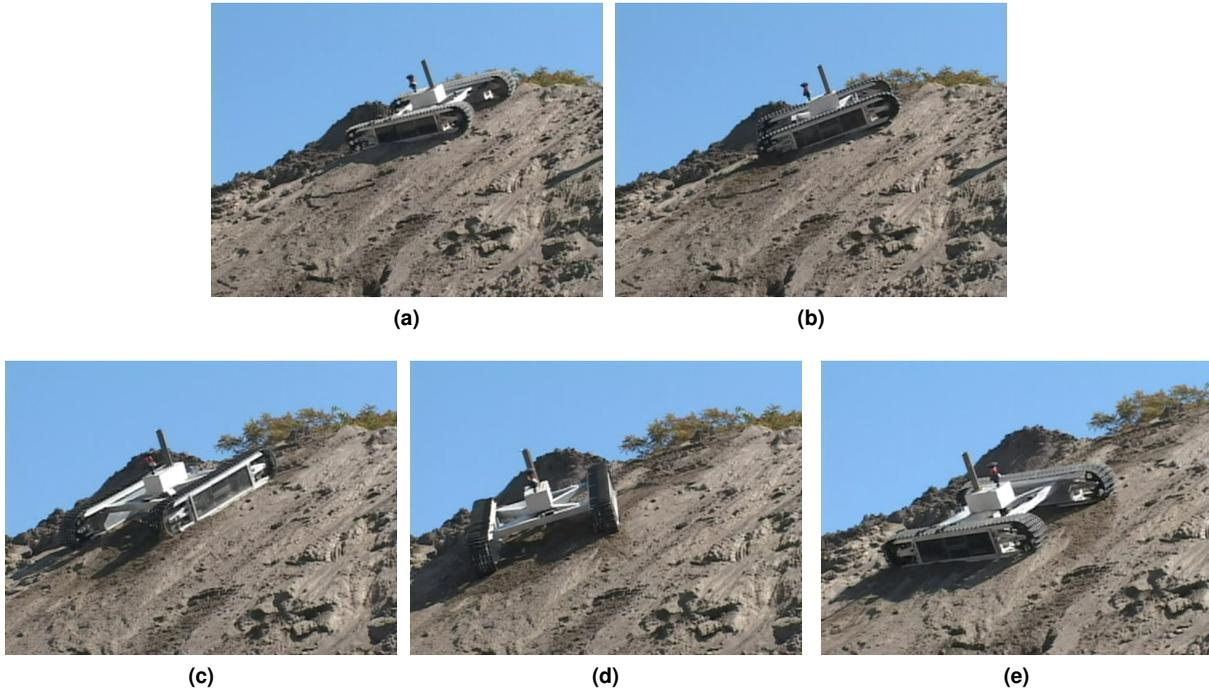
**Figure 3.** Sequence of rover orientations, showing a single trial of the turning test. For reference, the orange crystal is mounted towards the front of the rover.
