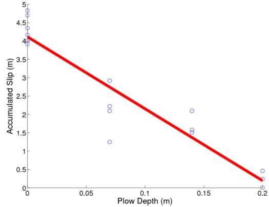
**Figure 8.** Slip rates during linear descent with various plow depths.
