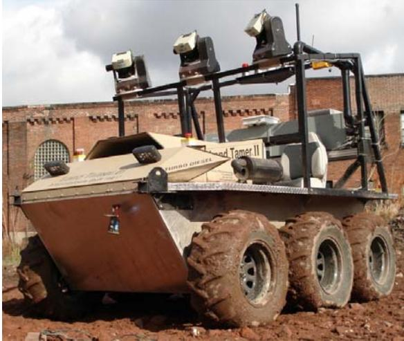
**Figure 9: Robot Vehicle.** A LandTamer® vehicle was retrofitted for remote control. Three custom colorized range (CR) sensors with a total field of view of 160° are mounted high on the vehicle looking forward. The lidars are manufactured by SICK providing range points at 13 KHz separated by ½ degree of angle over 180° of field of view. The cameras are the Firefly® by Pt. Grey Research Inc., and they provide color imagery at 720 X 500 resolution over a 60 degree field of view.
