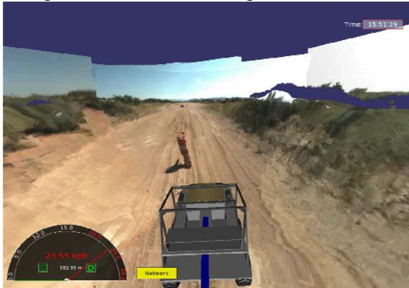
**Figure 18: High Speed Obstacle Avoidance.** Latency compensation is most valuable during high speed driving. Here, the operator avoids an obstacle by fitting the vehicle into a narrow space to its right. A custom fly-behind view was used. The speed reached approximately 24 km/hr. The operator control station is about 1 km farther down the road.
