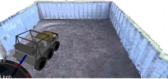
**Figure 14:** Legos. Projecting video onto small cubes at the correct range is an inexpensive way to visualize data whose surface shape cannot be resolved. Here, the vertical walls of trucking containers are very clear despite the inaccuracy of their local surface geometry.
