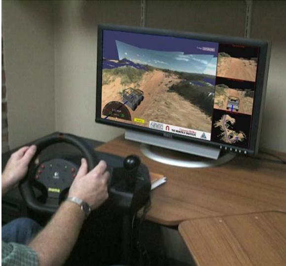
**Figure 10: OCS.** The Operator Control Station includes a steering wheel equipped with selection buttons. It also has foot pedals, and a large LCD display. The display provides selectable views including the raw video, over-the-shoulder, and bird's-eye (direct overhead).
