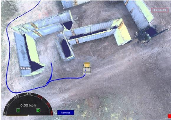
**Figure 20: Map of Maze Course.** This course was used to test the capacity of operators to solve a maze while conducting a search. This highly accurate photorealistic 3D model was produced from on-board perception and our visualization system.
