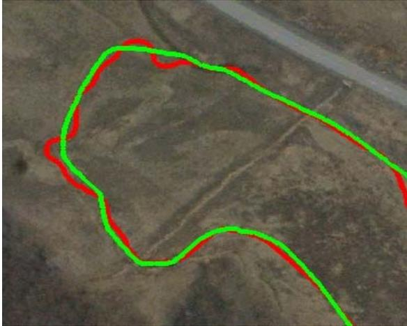
**Figure 3: Effects of Video Latency on Teleoperation Performance.** For even expert drivers, an increase in latency from 360 msec (green) to 1300 msec (red) doubles driving time, halves average speed and produces a system declared “impossible” to drive.
