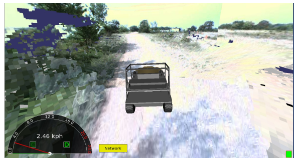
Figure 9. Projective texturing is a hardware-based alternative to texture-mapping that improves realism and efficiency.
