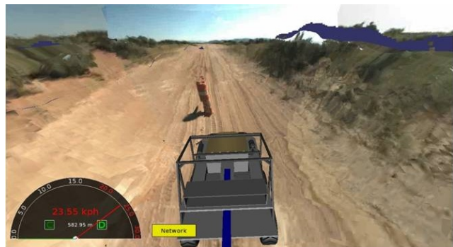
Figure 1. Our approach models 3D environments realistically and in real-time. The sensors used to capture this scene are mounted on the vehicle, which is shown using a synthetic representation, but we render the scene from an over-the-shoulder viewpoint to improve situational awareness for the tele-operator, who is avoiding obstacles while driving at 23 kph.
