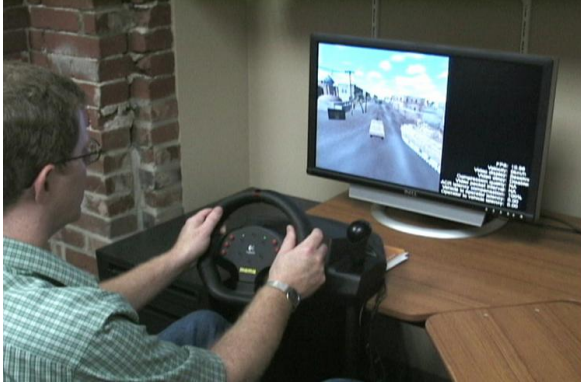
Figure 3. The operator control station allows the remote operator to steer the vehicle and control its speed while visualizing the environment from user-selectable viewpoints.
