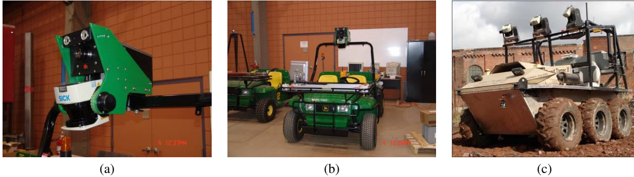
Figure 2. The video-ranging module (a) consists of a video camera and a nodding laser range-finder. The Gator (b) and LandTamer 2 (c) vehicles were retro-fitted for tele-operation and used in our experiments.
